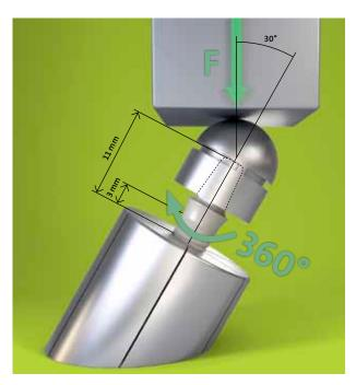
Fig. 1: Test setup according to ISO 14 801
